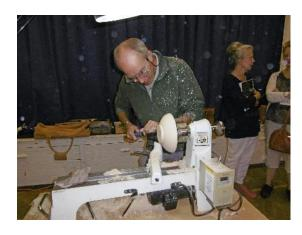
Mike mounted a piece of Sycamore on a screw chuck and started to shape the outside of a small bowl. He then reversed it into a four-jaw chuck and hollowed out the inside. He showed how you can, with good tool technique, get a good finish straight from the tool. The advantage of this is that it requires less sanding to get the final finish.
